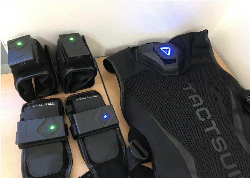
Figure 3. The vest, armor, and hand parts of BHaptics' X40 VR haptic suit
